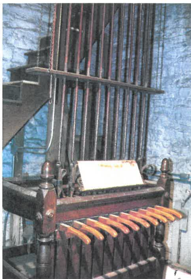
Interior view of the tower with levers controlling the chimes.
